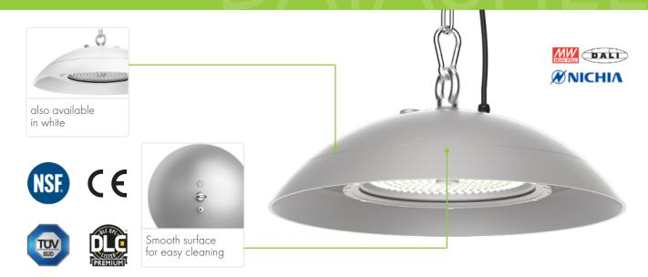
Very robust LED Highbay for the (food) industry with special requirements: NSF-certified, IP69K protection class (withstands strict highpressure and high-temperature washing procedures), IK10. Extremely high system efficiency with true 160 lm/W, long life, excellent thermal management. Smooth exterior, no exposed fasteners. Impact-resistant, shatterproof PC (polycarbonate) diffuser in accordance
