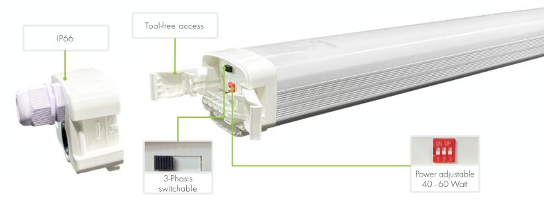
Highly efficient LED triproof (moisture-proof luminaire) for use in extreme operating environments: bright, robust (IK10) and jet-proof (IP 66). Impact-resistant, shatterproof cover made of PC (polycarbonate) in accordance with the requirements of the International Featured Standard Food (IFS Food).
